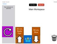
34. In the workspace, Repeat has two blocks that are next to each other (you may have to scroll left or right to find both). The one on the left is Repeat and the one on the right is End Repeat. We can put the commands we want to repeat in between these two blocks (*inside the loop*).
